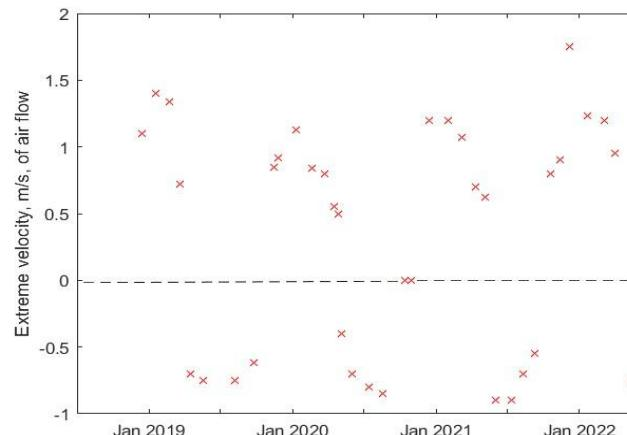
In winter the maximum outflow velocities varied 0.50...1.75 m/s. Typical air outflow is 300 m³/h, with H₂O content 2.5 kg/h.
